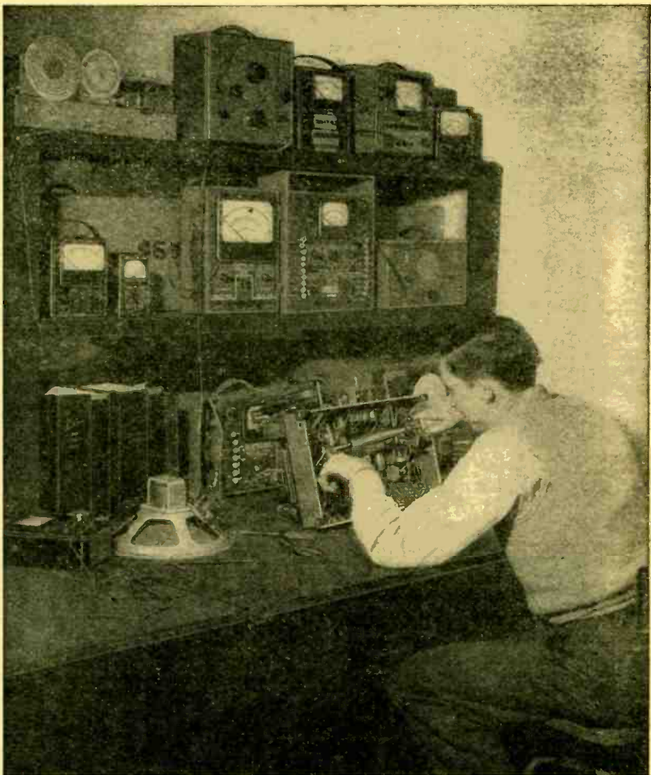
Work on the new Sams' test bench. Left portion is part of a second identical bench used to double length. The large stock of meters represents part of Sams' equipment-testing program.
